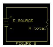
c. Notice that this single resistor has the same total resistance, same current and same voltage as the original series-parallel circuit in Figure 1. Why, then, could you not use this one resistor to complete all of the procedures in this experiment?
