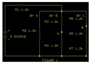
2. With the current meter in series with the entire circuit, set the supply voltage so that the current meter reads exactly <u>6 ma</u>. Measure the source voltage and record.
