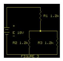
b. Change  $R_2$  to a value of 2.2 k $\Omega$ . Repeat procedures 1 through 5. Record in Table 4.
